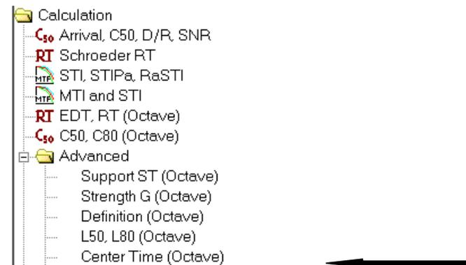
Then the graph Center Time is shown using the octave-filter midband frequency.
