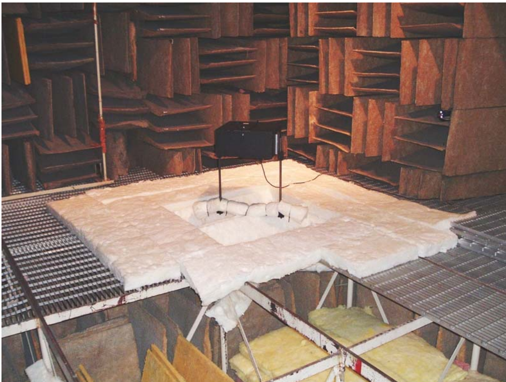
Photo 7 – Absorption on non-removable floor grates and in the well housing the turntable
